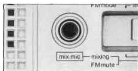
24. Mixing microphone socket When microphone (of low impedance) is connected to this socket, the sound entering this microphone are amplified and played through speakers or recorded and mixed with the signal from one of the following units, such as the built-in radio, record player, or other audio unit connected to line input sockets.
