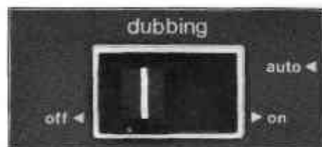
23. Dubbing switch For dubbing from Deck 1 to Deck 2, put this switch to the ON position. This switch prevents any recording through the built-in microphone after Deck 1 has automatically stopped.
